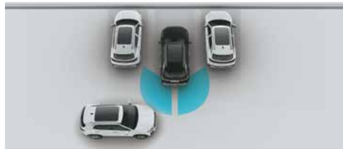
Rear Cross - Traffic Collision - Avoidance Assist (RCCA) & Rear Cross - Traffic Collision Warning (RCCW)
